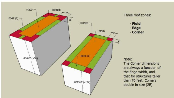
these zones and provide a width for the edge zone. The width of the edge is never static, and always a function of building geometry, but will never be less than 2.0 m (7'). These wind load values are the key to
