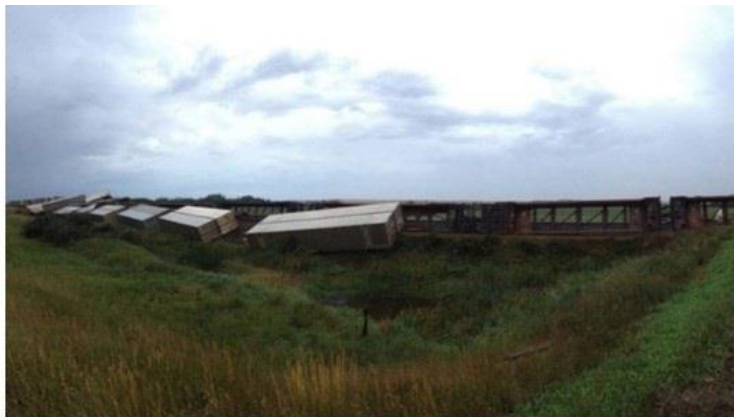
Plow winds, blowing 70 km/h, derailed this train near Waldeck, SK (2014)
