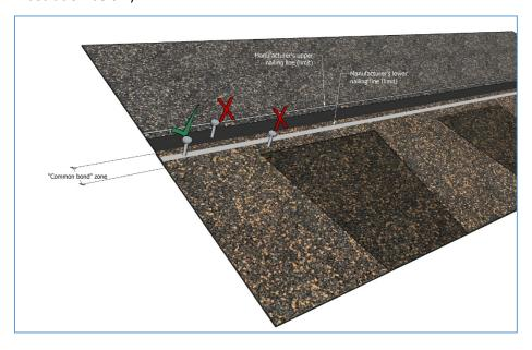
Securing asphalt shingles through the common bond is a well-established RGC standard, and it is supported by the more recent CSA Standard for asphalt shingle application (CSA-A123.51):
