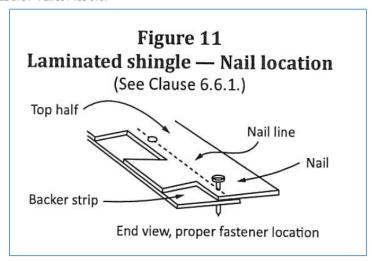
The reasoning behind the RGC requirement is simple: shingles stay put when they are nailed through the laminated region. Nails installed above the common bond risk shingle detachment and product failure.
