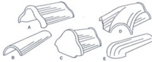
Figure 1-2 High Profile accessory tiles (A) ridge (B) hip (C) closed ridge end (D) terminal (E) gable terminal.
